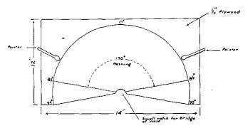
FIGURE 33.- Equipment for field of vision test.
